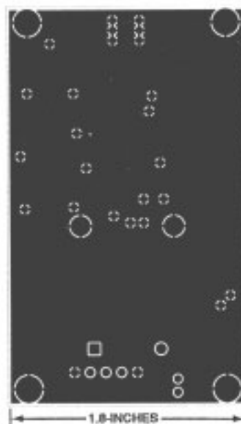
Here's the foil pattern for the solder side of the printed circuit board. Connecting the ground planes on both sides of the board to each other is important for proper operation.
