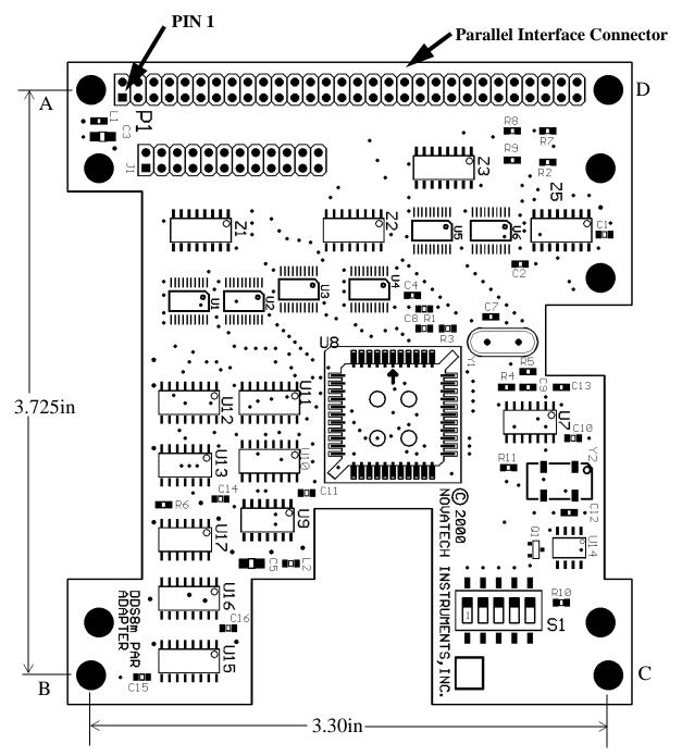
DDS8par Parallel Adapter Component/Connection Location Diagram (Not to Scale)
