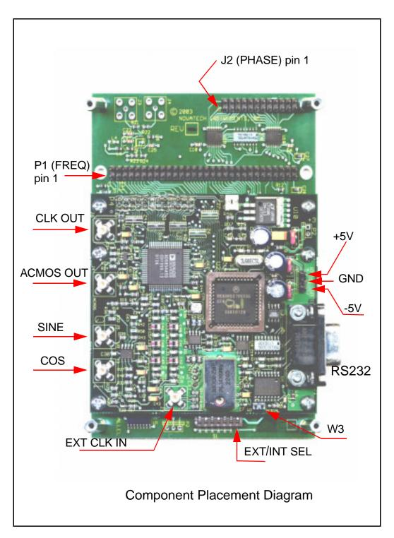
**Hardware Mounting:** The DDS8m synthesizer module is attached to the DDS8p parallel adapter board using 6 aluminum spacers and 12 screws. These must remain undisturbed. There are 6 free mountings holes with clearance for 3mm or #4 screws. The mounting hole pad is connected to Circuit Common (ground). It is suggested that all 6 positions be used to attach board into the application. Please leave approximately 3mm clearance spacing from the bottom of the board.
