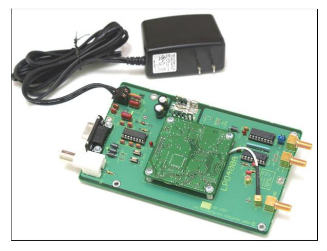
The LPO400A evaluation board is similar to the 440A, but is supplied without a case to make evaluation of the LPO400A module easier. See the schematic below for details on the board.
