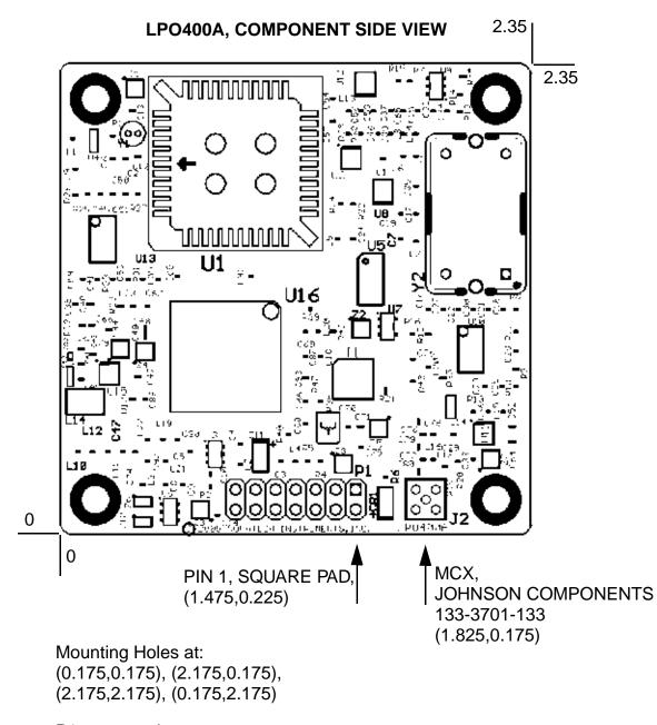
P1 two rows by seven pos., on 0.1 (2.54mm) grid.
